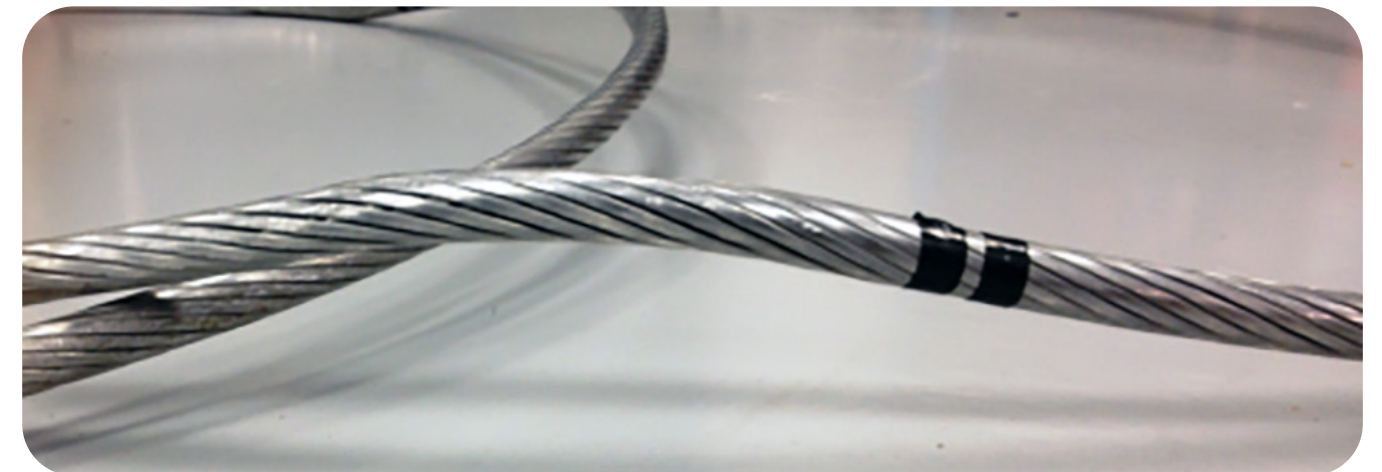
Figure 5: If the conductor has taken a "set" from bending, the bent section should be cut out and a full tension splice installed.
