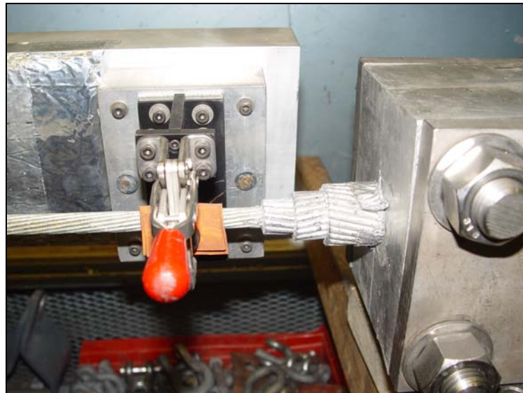
Figure 2, Typical Resin Socket and Extensometer
