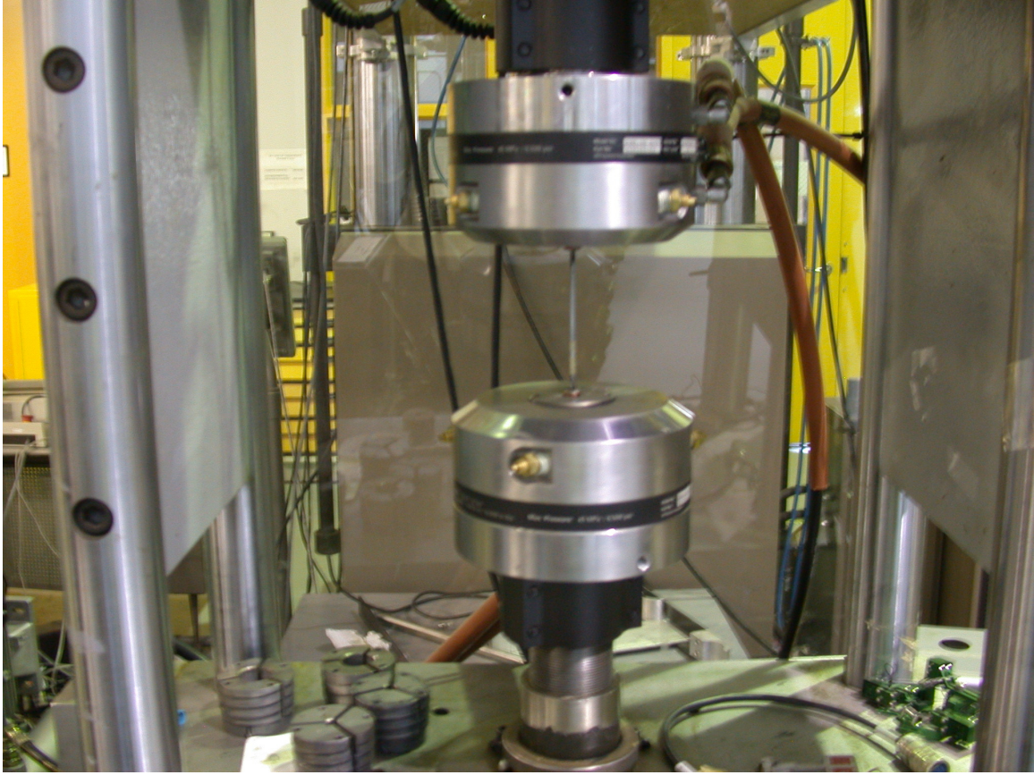
Figure 1 shows the test setup. Wire is gripped between the upper and lower grips. The upper grip is fixed while the bottom grip rotates.
