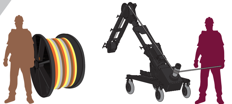
Wire pulled with Maxis® XD10 EXTREME Duty Cable Puller by 2 people.
