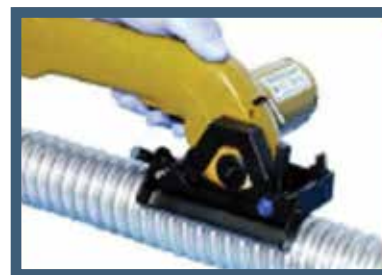
Using motorized saw to cut armor sheath to cut two adjacent convolutions on armor between 1.8 & 5 inches
