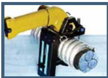
Motorized saw cuts armor and conductors
