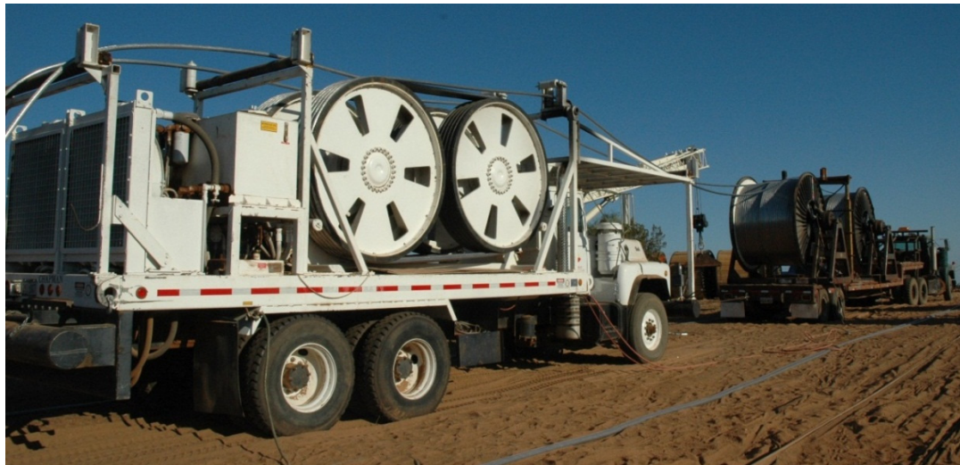
Figure 7. Dual drum bullwheel, courtesy of Oncor.
