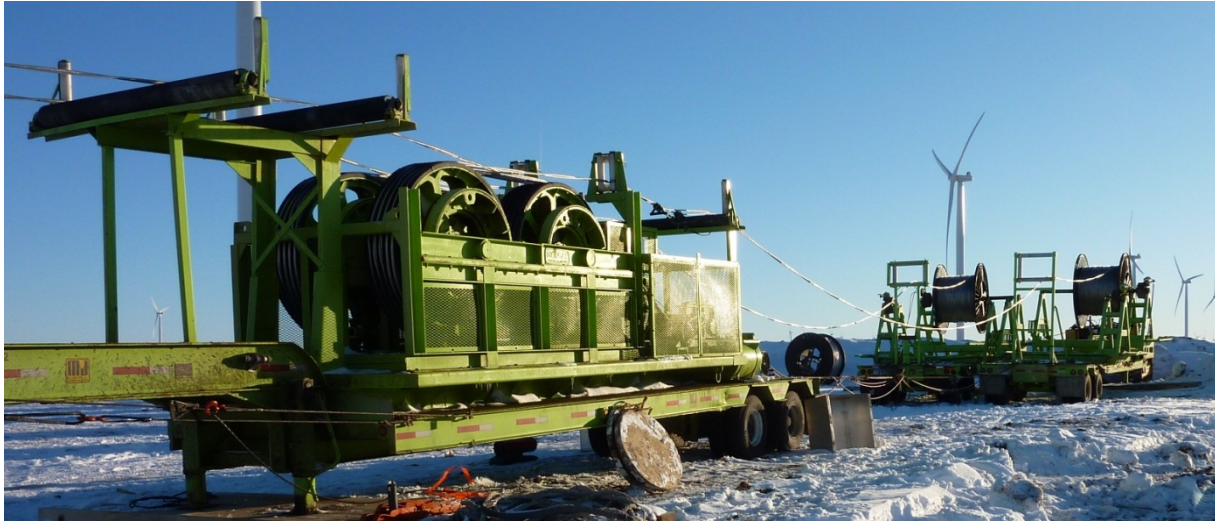
Figure 9: Payoff and bullwheel setup.
