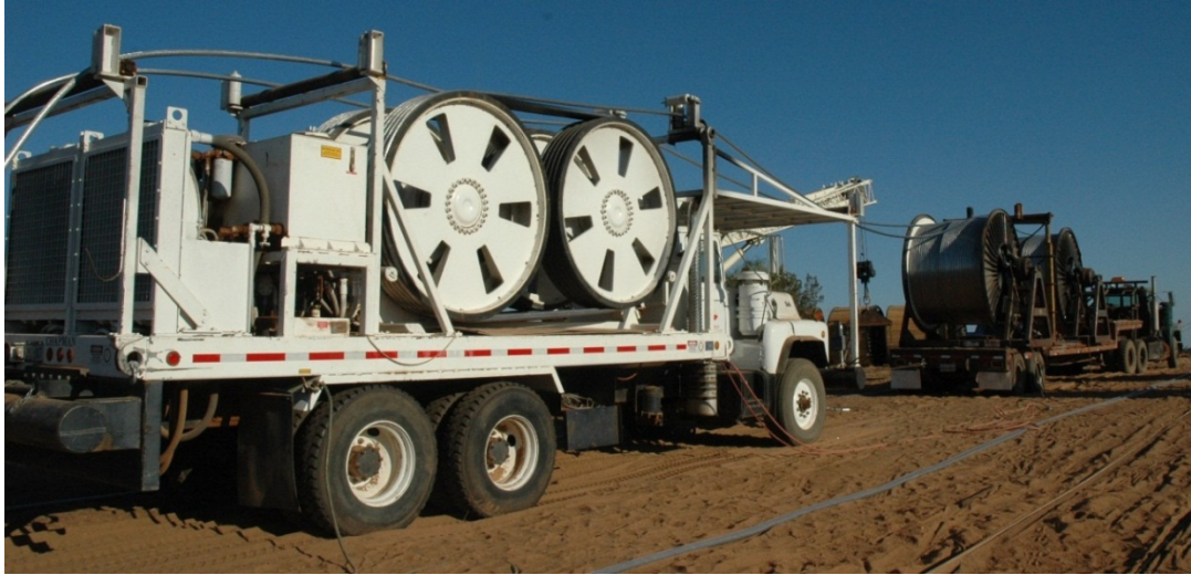
Figure 8. Dual drum bullwheel, courtesy of Oncor.
